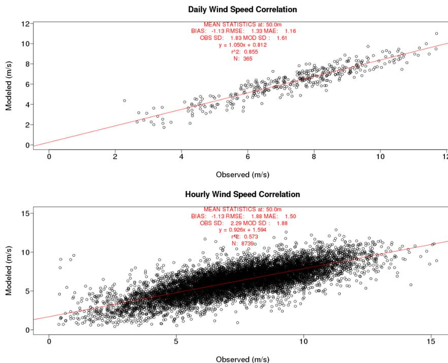
**Figure 1a.** Scatter plots of observed and WRF daily average (top) and hourly average (bottom) wind speeds at the Bovoni2 tower for 2013.
