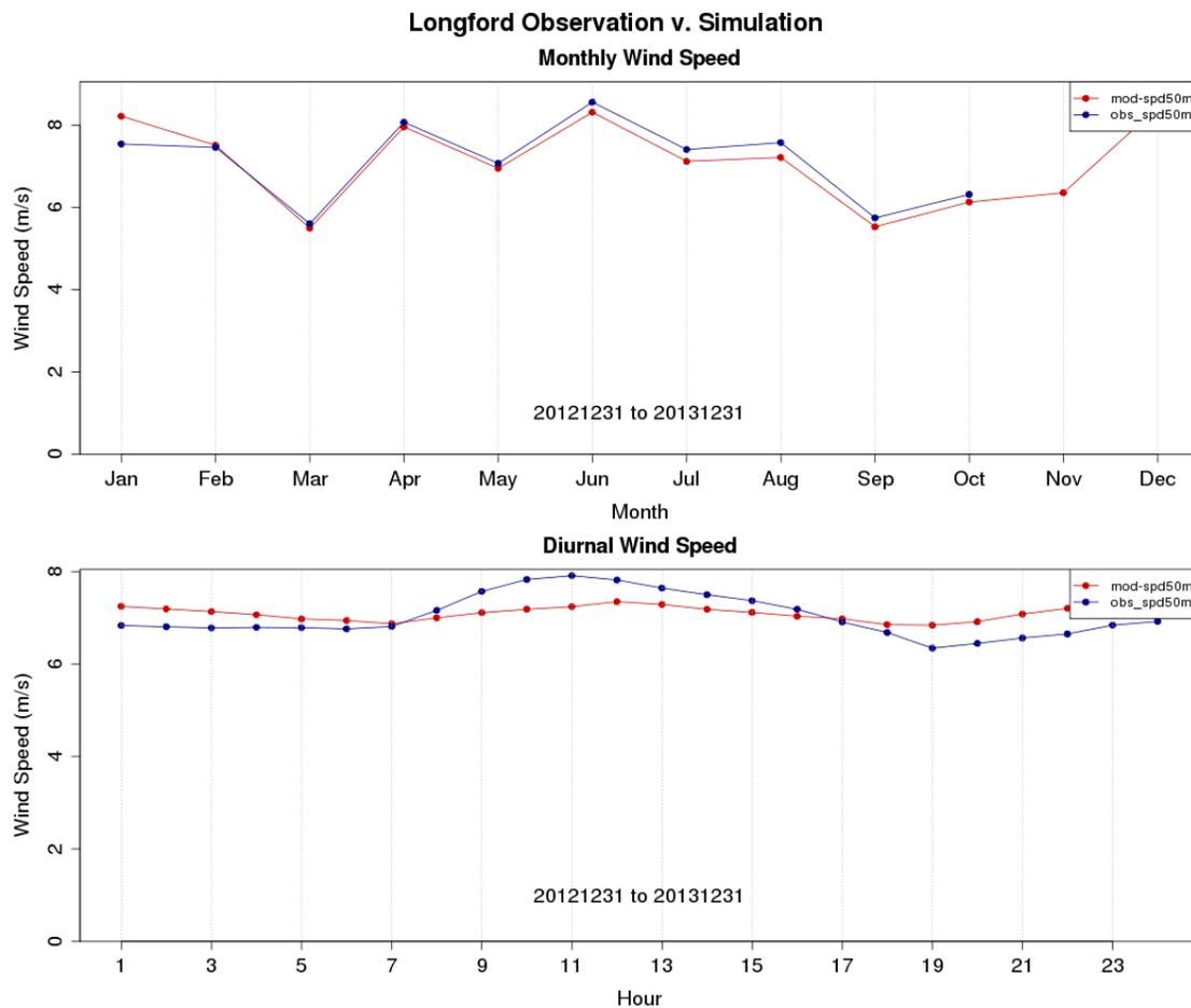
**Figure 2c.** Comparison of observed and WRF-generated monthly average (top) and diurnal average (bottom) wind speeds at Longford.
