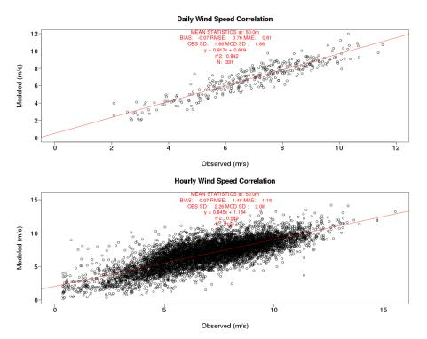
Figure 2a. Scatter plots of observed and WRF-generated daily average (top) and hourly average (bottom) wind speeds at the Longford tower for 2013.
