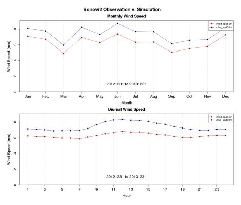
Figure 1c. Comparison of observed and WRF-generated monthly average (top) and diurnal average (bottom) wind speeds at Bovoni2.
